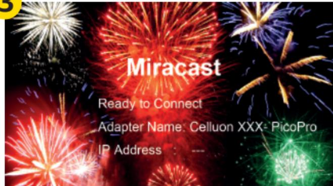
3. After about 20-30 seconds, "Ready to Connect" screen for Miracast will display.
