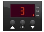
A red dot will appear next to "CD-L" when the press is closed. This indicates that the timer has started and is now counting down.
