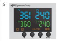
The "COUNTER" on the bottom right shows the number of transfer cycles. It can range from 0 to 999. Press "Reset" for 5 seconds to make counter go to 0.
