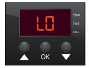
Press "OK" to enter real time mode. Note that the display might say "LO". This is because the heat press is still heating up.
