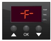
Press "OK". Use "▲" or "▼" to switch between "C°" or "F°" for your desired temperature scale.
