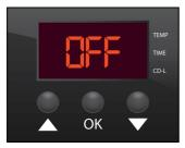
Turn on the power switch. It will say OFF. Press OK to turn on the machine. This is a safety feature. 2
