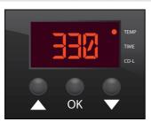
Press "OK" to set the temperature. A red dot will appear next to "TEMP". Use the arrow keys to select desired temperature.
